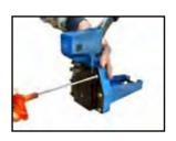
LOOSEN SCREWS (508) WITH 4 MM HEXAGON WRENCH KEY.
